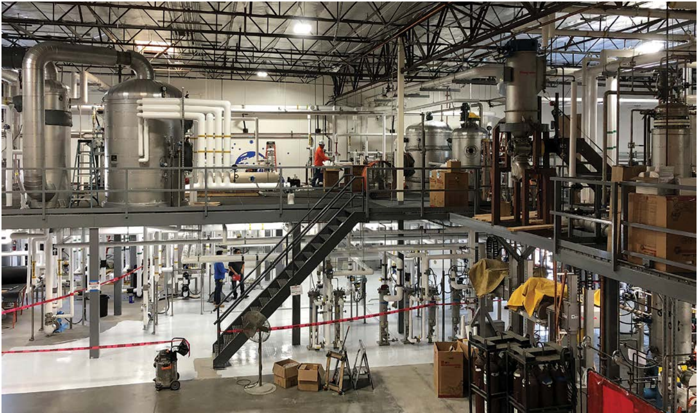
A modern small scale, 2000kg/hour, physical refining plant. Image courtesy of Dr. Bronner in the USA
